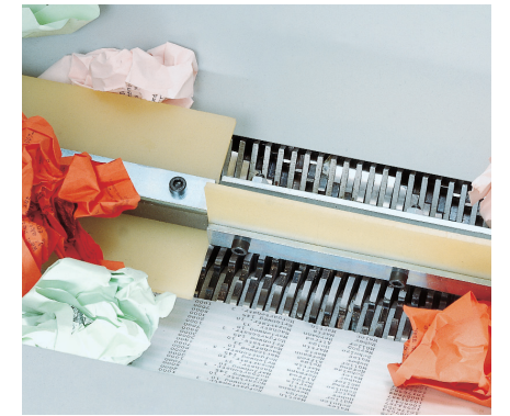
BULK PAPER SHREDDING (4606) Special rotating paddles are used to feed bulky materials into the cutting unit.
