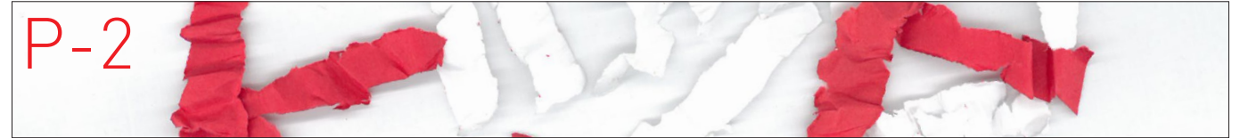
Material particle surface \leq 1.25 " squared or strip width \leq .25 ". Strip length not determined.
