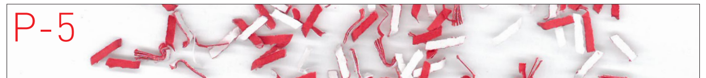
Material particle surface \leq .468 " squared and for regular particles: strip width \leq 3/32 " ( 3/32 " x 5/8 " particles, for example).
